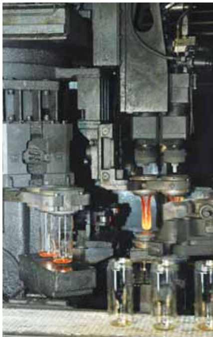
▲ The picture shows a parison, that, in order to reach its final form, has to be transferred to the mould. On the left hand side and in the foreground ready-blown glasses can be seen.
