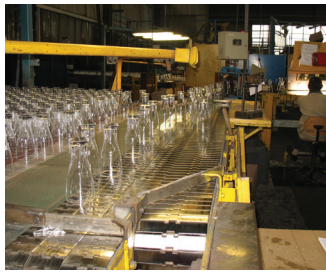
▲ Vibration plate with single liners.
