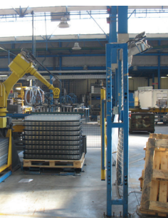
▲ The glasses, directly from production or decoration, are collected by the main robot and are put in their place in the box.
