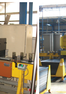
▲ The glasses, directly from production or decoration, are collected by the main robot and are put in their place in the box.
