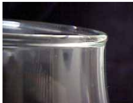
Fig 1 - Typical burn-off rim
