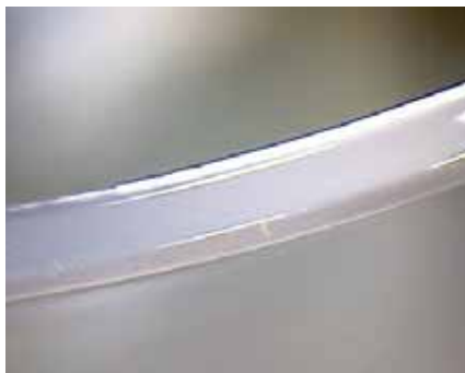
Fig 6 - High end cold cut glass showing accurate bevel.
