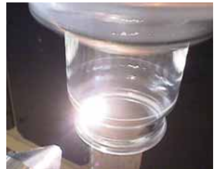
Fig 4 - Biebuyck laser Generation 2 cold cutting
