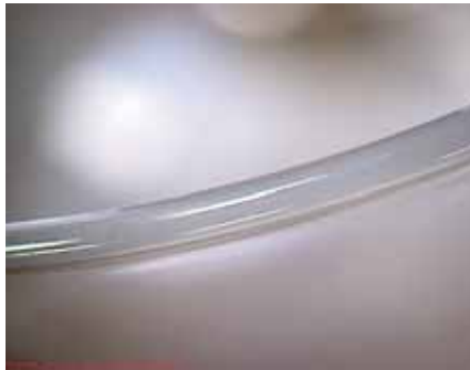
Fig 5 - Regular cold cut edge.
