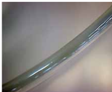
Fig 3 - Federal style but laser cold cut with direct fire polishing
