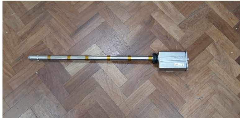
NIR-b-2k camera, 2ft probe, range 1000-1800C.
