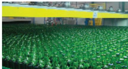
▲ Fig 3. Bottles at the exit of the annealing lehr tunnel.
